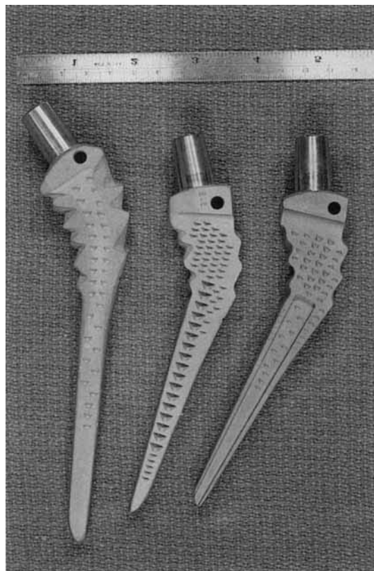
Fig. 2. BMO- (biomechanically optimized-) Stepped Stem of the femoral component of the FRIALIT total hip replacement system made of the vanadium free TiAlFe alloy. Note the macroscopic steps and additional fine surface undulations providing for an interlocking along otherwise tangentially loaded interfaces.
